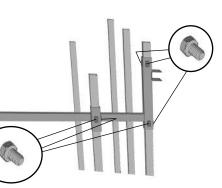
**7e.** Adjust upper main arm end up or down the 48" 3rd tier arm for desired height for 3rd tier. *It is recommended* that the rear top of the upper main arm end is flush with the top of the 79" vertical post.
