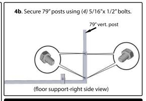
NOTE: After securing/bolting both sets of the vertical posts to the floor supports, there WILL BE PLAY in the vertical posts and bottom base assembly until the main arms and top rails are attached.
