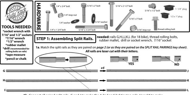
**1b.** Connect all paired split rails--G and J to make the 4-2nd and 3rd tier top rails, H and K to make the rear bottom rail, and I and L to make the front bottom rail.
