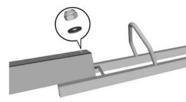
**3d.** Fasten bolt/washer in place using a 1/4" washer and 1/4" stop nut. Tighten LOOSELY using both the 7/16" socket/wrench and 7/16" wrench.
