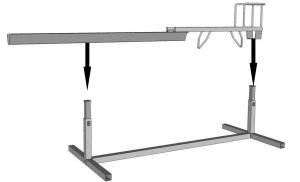
**1i.** Line up remaining holes in tray assembly with the HL inserts.
