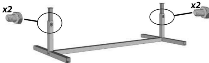
**1d.** Turning the tray and stanchion upside down, line up the holes on the trays to the stanchion.
