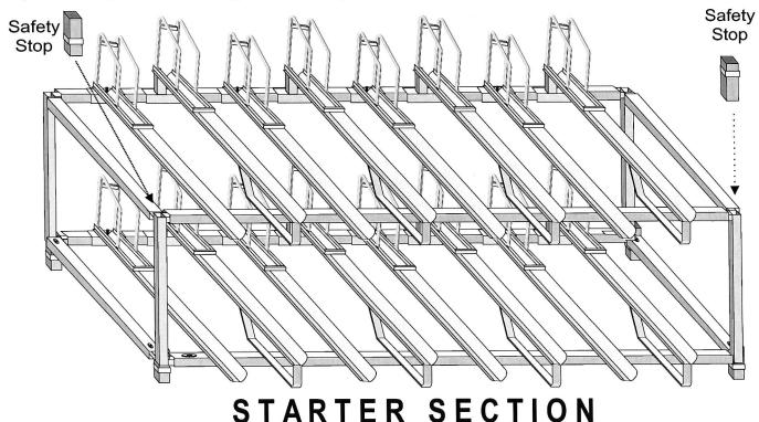
**NOTE:** The Wall Double Decker shown here has 8 trays per tier. You may have a section with more or less trays. Follow these instructions, putting the appropriate number of trays on to each section of the rack.
