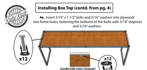
**NOTE:** Tighten each bolt/washer/nut combo gradually, working your way around the surface as done with the corner frame assembly. DO NOT OVER TIGHTEN.
